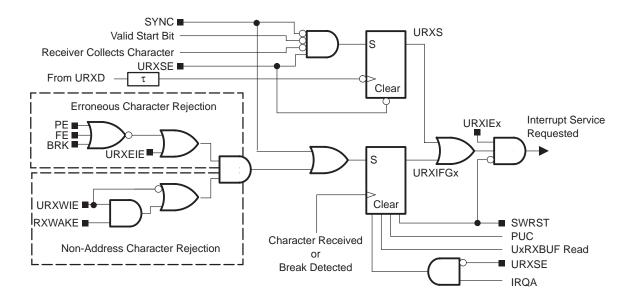
URXEIE is used to enable or disable erroneous characters from setting URXIFGx. When using multiprocessor addressing modes, URXWIE is used to auto-detect valid address characters and reject unwanted data characters.
